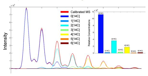
TrueCal calibration on both high and low resolution instruments enables powerful quantitative mixture deconvolution never before possible on any MS by utilizing the patented TrueFit RX™ technology. The above graph illustrates the accurate quantitative analysis of a drug compound containing a [14C] radio-labeled aromatic ring with up to 6 substitutions.
