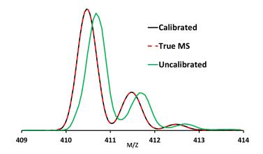
CLIPS (Calibrated Line-shape Isotope Profile Search) combines unsurpassed mass accuracy with the highest Spectral Accuracy to get the most out of your quadrupole MS.
