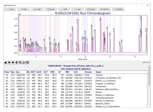
GC/ID processes an entire run in a few minutes and calculates the NIST match value (NIST) for each peak, verifies the compound formula ID by accurate mass/spectral accuracy (SA-M) as well as fragement ions (SA-F) and then calculates the peak's retention index (RI Fit). **These additional metrics can dramatically improve compound identification confidence.**
