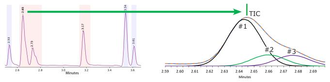
The peak at 2.65 min actually contains 3 co-eluting peaks which GC/ID deconvolves as shown.
