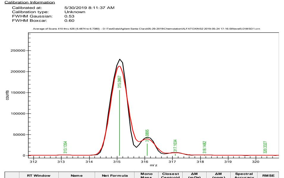
A single ion calibration using aflatoxin B2 (m/z 315) from the highest of 5 concentration levels was performed with MassWorks software through the full mass spectral calibration process published elsewhere<sup>2</sup>, resulting in the calibration review/report shown on the left and indicating excellent mass accuracy error of less than 1mDa and Spectral Accuracy of better than 99%
