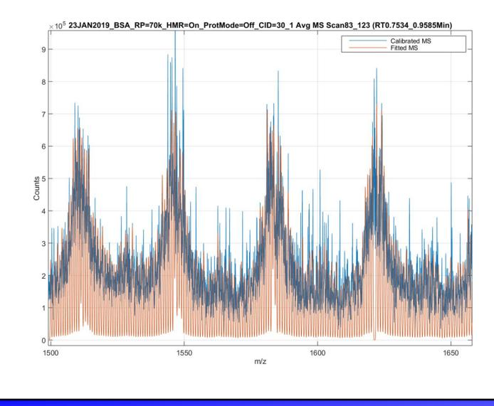
A mass spectral accuracy analysis on the left shows a section taken from z = 34-45 and in consideration of the many forms of K adducts. As can be seen, only about 60% of the observed mass spectral signal was accounted for by the postulated species. This research is currently on-going with the aim of revealiing what exactly gets formed under intact conditions in order to achieve the same level of high spectral accuracy expected of a pure single charge standard at similar signal-to-noise level.
