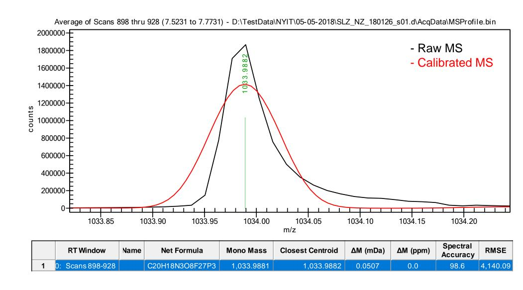
A full spectral calibration with MassWorks software tool allows for the TOF peak shape to be calibrated into a known functional form and thereby calibrating for both mass (m/z) accuracy and spectral accuracy. The spectral accuracy achieved is 98.6%, indicating the possible mass spectral residual error of about 1.4% at this (averaged) signal level.
