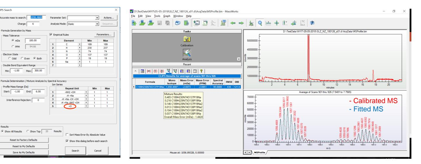
In order to account for the mass spectral signal around 1059.5 Da, it was postulated that possible oxidation may exist and the mixture analysis repeated with +O as an additional modification, resulting in improved spectral accuracy of 95.7% with the identification of this biochemically plausible modification and its relative quantitation (3.7%).
