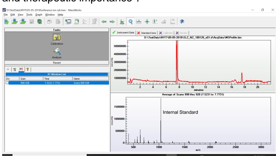
A 20-nt RNA measured on Agilent LCqTOF instrument with an internal single charge reference standard contained in the mobile phase at m/z 1034.
