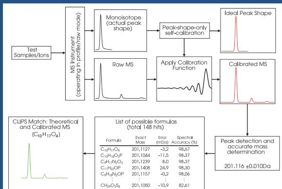
**Figure 3** • Flow diagram depicting the sCLIPS calibration and formula determination process. The entire process is automated into a single operation in the MassWorks software.
