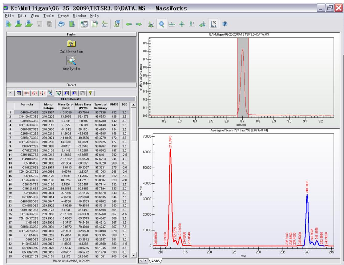
**Figure 4.** Averaged MS (Red) for the two large ions/fragments from the unknown at RT=8.7min and the theoretical MS for  $\text{C}_4\text{H}_8\text{N}_4\text{O}_4\text{S}_2$  (Blue).
