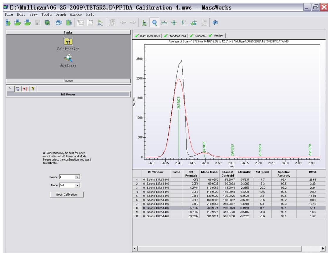
**Figure 3.** The raw (black) and the calibrated (red) mass spectrum for the PFTBA calibration fragment ion  $\text{C}_5\text{F}_{10}\text{N}^+$  (exact mass 263.9871Da).
