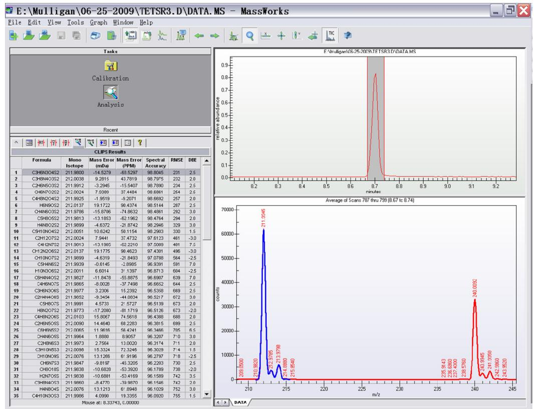
**Figure 6.** Averaged MS (Red) for the two large ions/fragments from the unknown at RT=8.7min and the theoretical MS for C<sub>3</sub>H<sub>6</sub>N<sub>3</sub>O<sub>4</sub>S<sub>2</sub> (Blue).
