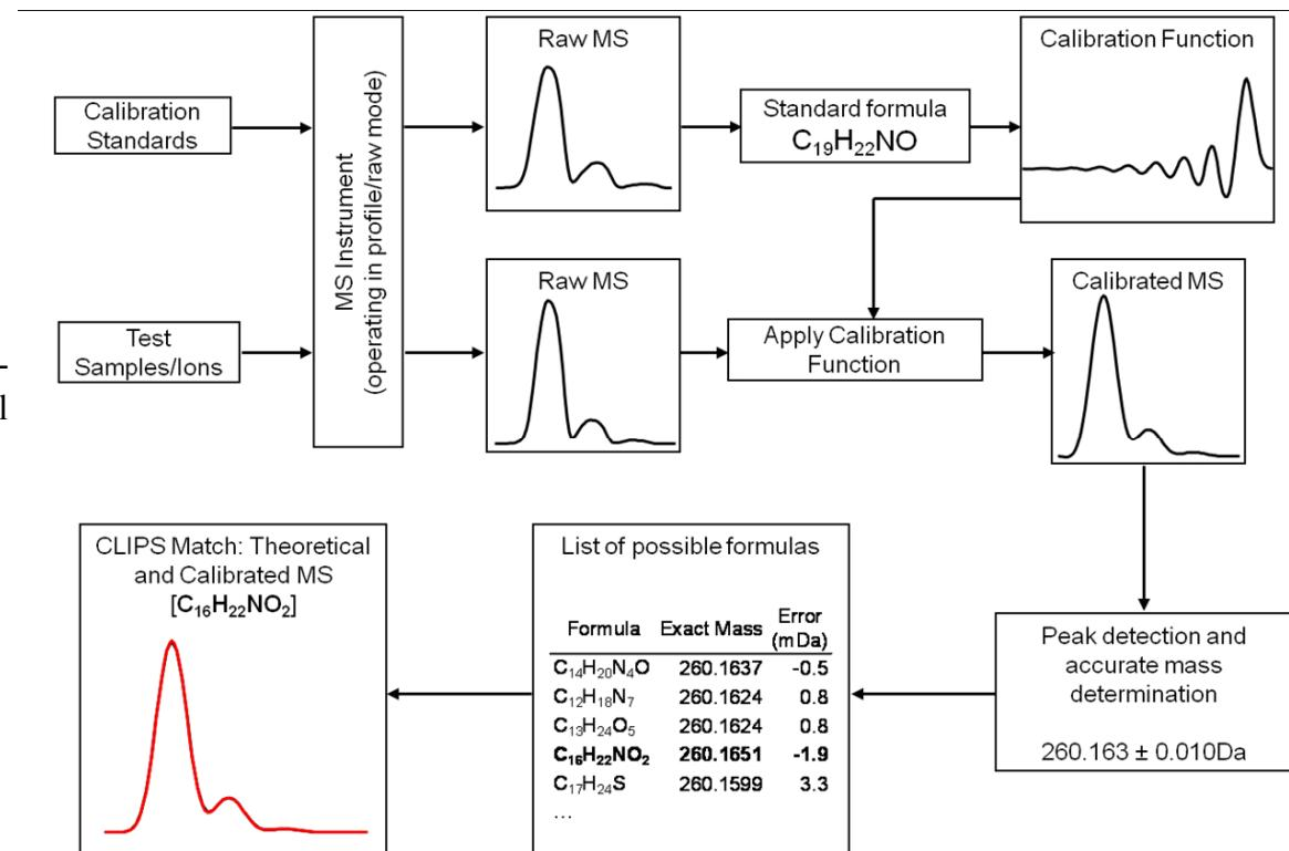
**Figure 2.** The general flow of MassWorks calibration and its elemental composition determination process.
