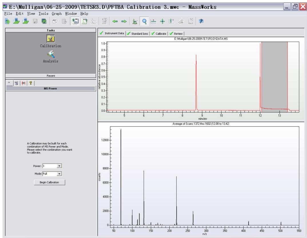
**Figure 1.** TIC (top) and the average PFTBA calibration spectrum from a single GC/MS acquisition (bottom).
