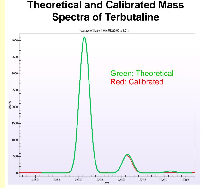
What is interesting is that the observed isotope pattern of Terbutaline have normal distribution for monoisotope (M) and 13C peaks (M+1), but a large portion of (M+2) peak is missing. In this case, sCLIPS search for m/z 226 achieved high spectral accuracy of 98.2% using isotope peaks of M and M+1 only.
