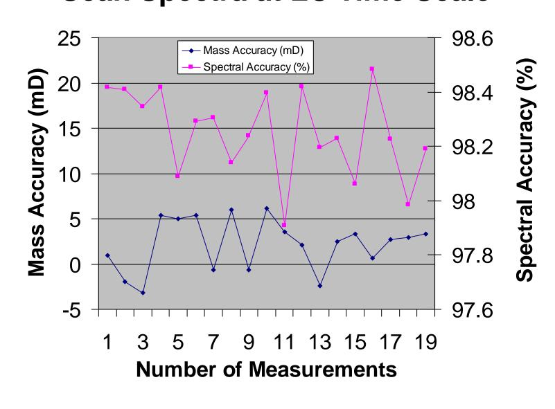
The zoom scan spectra of Terbutaline averaged for 3 seconds have mass accuracy better than 10 mDa and spectral accuracy better than 98% for all the 19 measurements. These results indicate the zoom scans can be used for LC/MS data acquisition for the purpose of accurate mass measurements and formula identification.
