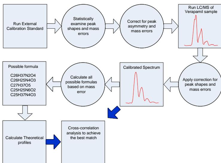
Figure 1. Data processing work flow for profile searching
