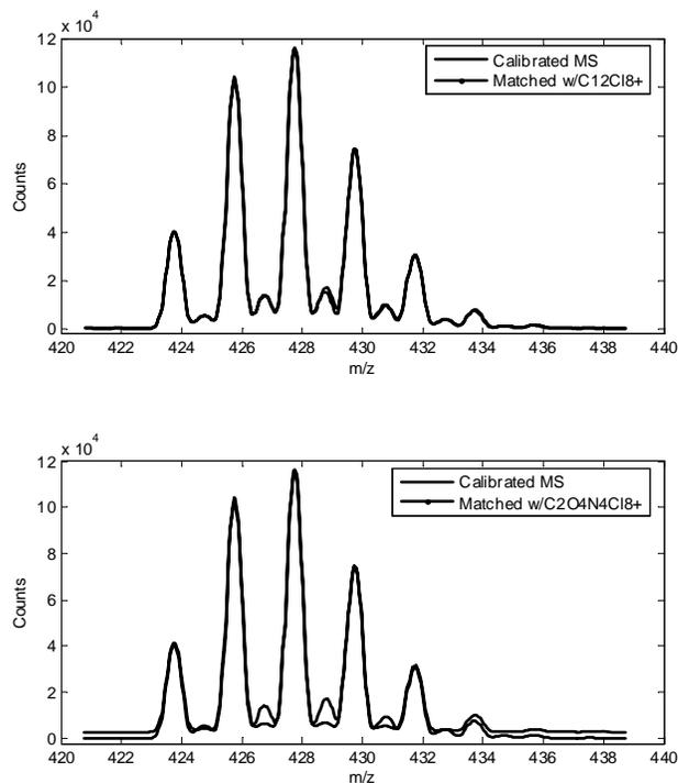
Figure 4. Isotope matching for the 1st (top) and 17th (bottom) hit from the elemental composition search on monoisotope masses.
